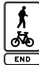
End shared path sign
