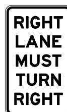
Right lane must turn right sign
